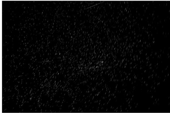
(b) Image after HSV filtering and binarization
